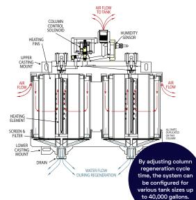
Because of this feature, the Dual Column Breather helps ensure an uninterrupted supply of dry air. Unlike competitive breathers that have a capacity limit, the Dual Column Breather has the ability to regenerate and still breathe, without the need for "quiet" time. This means the Dual Column Breather has the capacity to support virtually any application.
