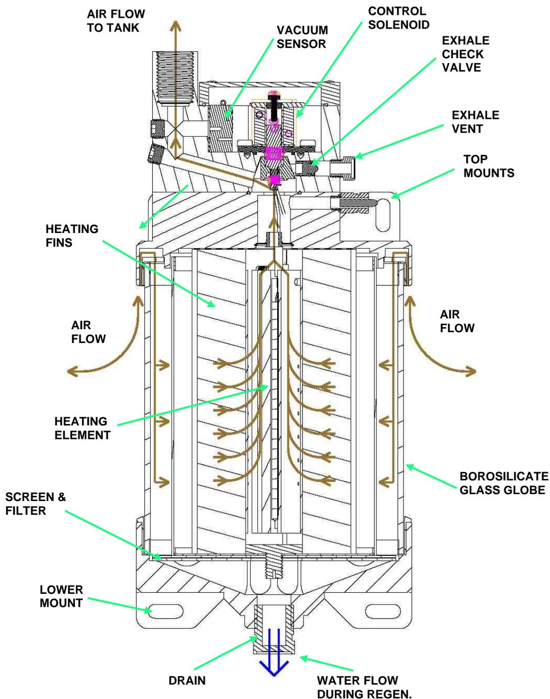
**Figure 1 – Standard Single Column Breather (SCB) Functional Operation and Component Identification.**
