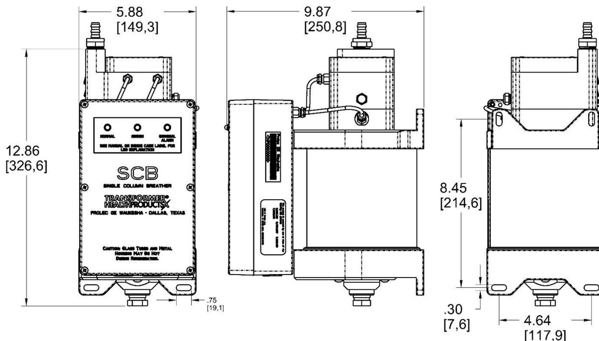
1. Measure and mark mounting holes or studs as shown by the center-to-center distances in Figure 2 above.
